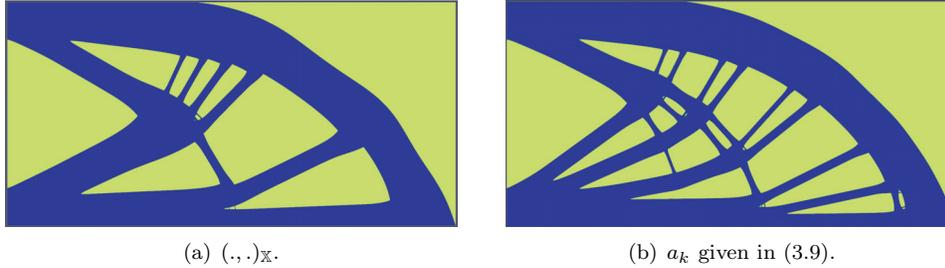
FIG. 1. Local minima for the cantilever beam.
